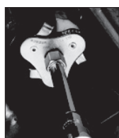
Adjustable oil filter wrench
